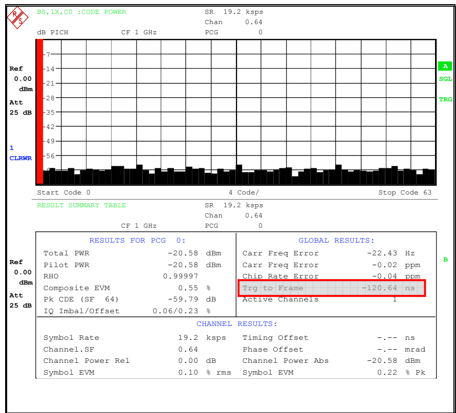
Fig. 4.2.1.1.2 - Pilot Timing Tolerance measurement result
